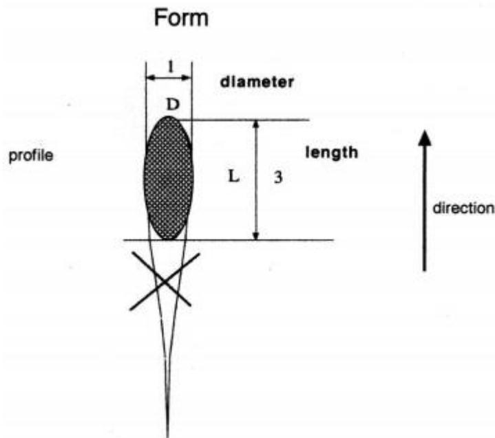
A fuselage form shall be defined as an extension or streamlining of a section. This shall be tolerated as long as the ratio between the length L and the diameter D does not exceed 3. This rule does not apply to frame and fork of the bicycle.
